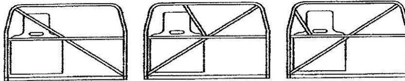
ADDITIONAL BRACING BEHIND DRIVER'S HEAD IN MAIN HOOP REQUIRED.
